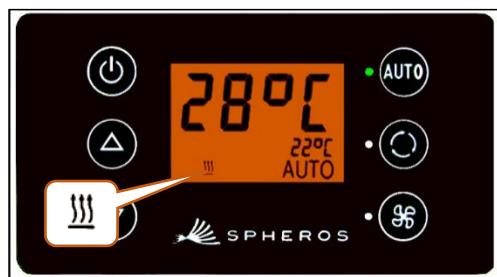
Figure 8 - SC600 Auto mode activated, Heating mode
