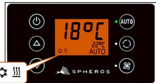
Figure 11 - SC600 dehumidify activated
