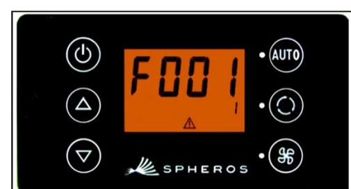
Figure 14 - SC600 Error detection mode
