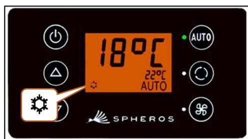
Figure 7 - SC600 Auto mode activated, Cooling mode
